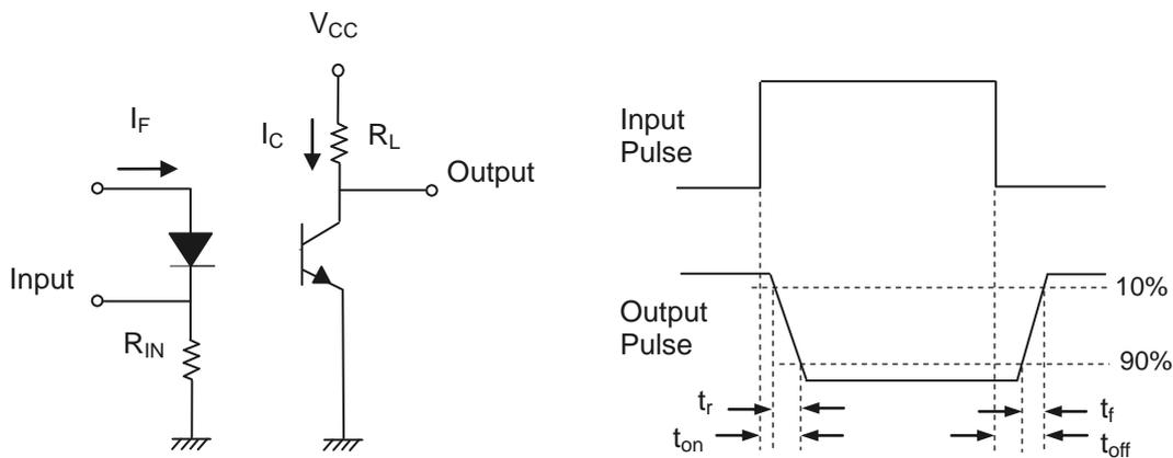
Figure 10. Switching Time Test Circuit & Waveforms
