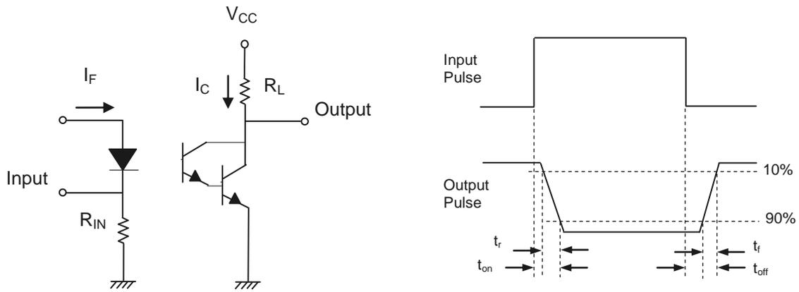
Figure 7. Switching Time Test Circuit & Waveforms
