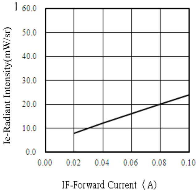
Fig.4 Relative Radiant Intensity vs.
