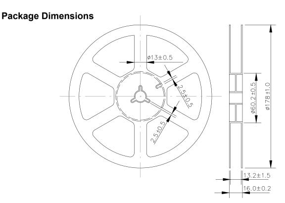
**Note:** The tolerances unless mentioned are ±0.1 mm, unit: mm.
