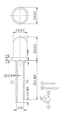
Note: Tolerances unless dimensions ±0.25mm
