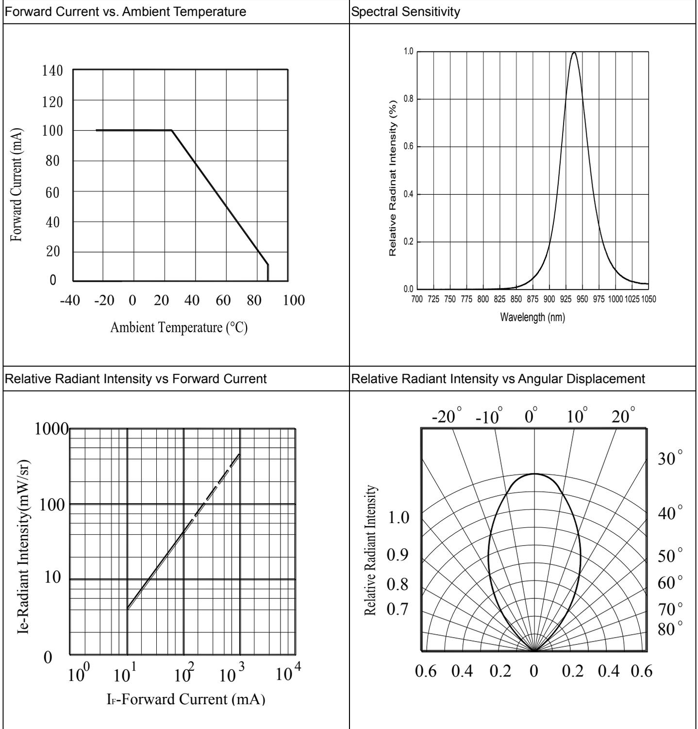
**Typical Electrical/Optical/Characteristics Curves for PT**
