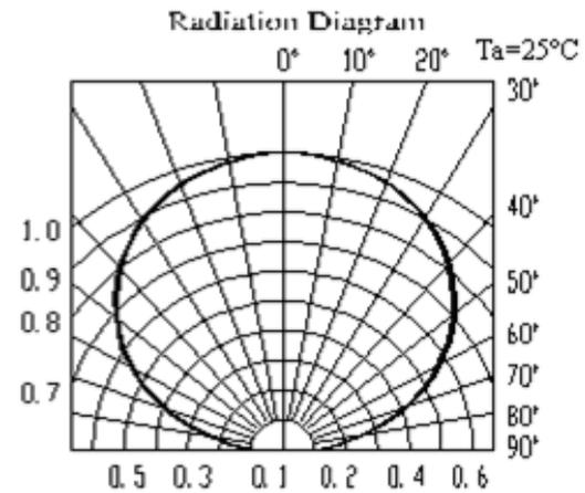
**Typical Electro-Optical Characteristics Curves**
