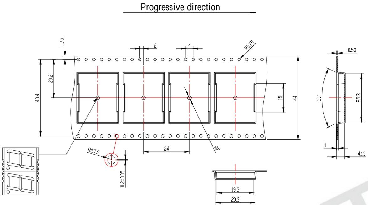
Note: Tolerances unless mentioned  $\pm 0.25$ mm. Unit = mm
