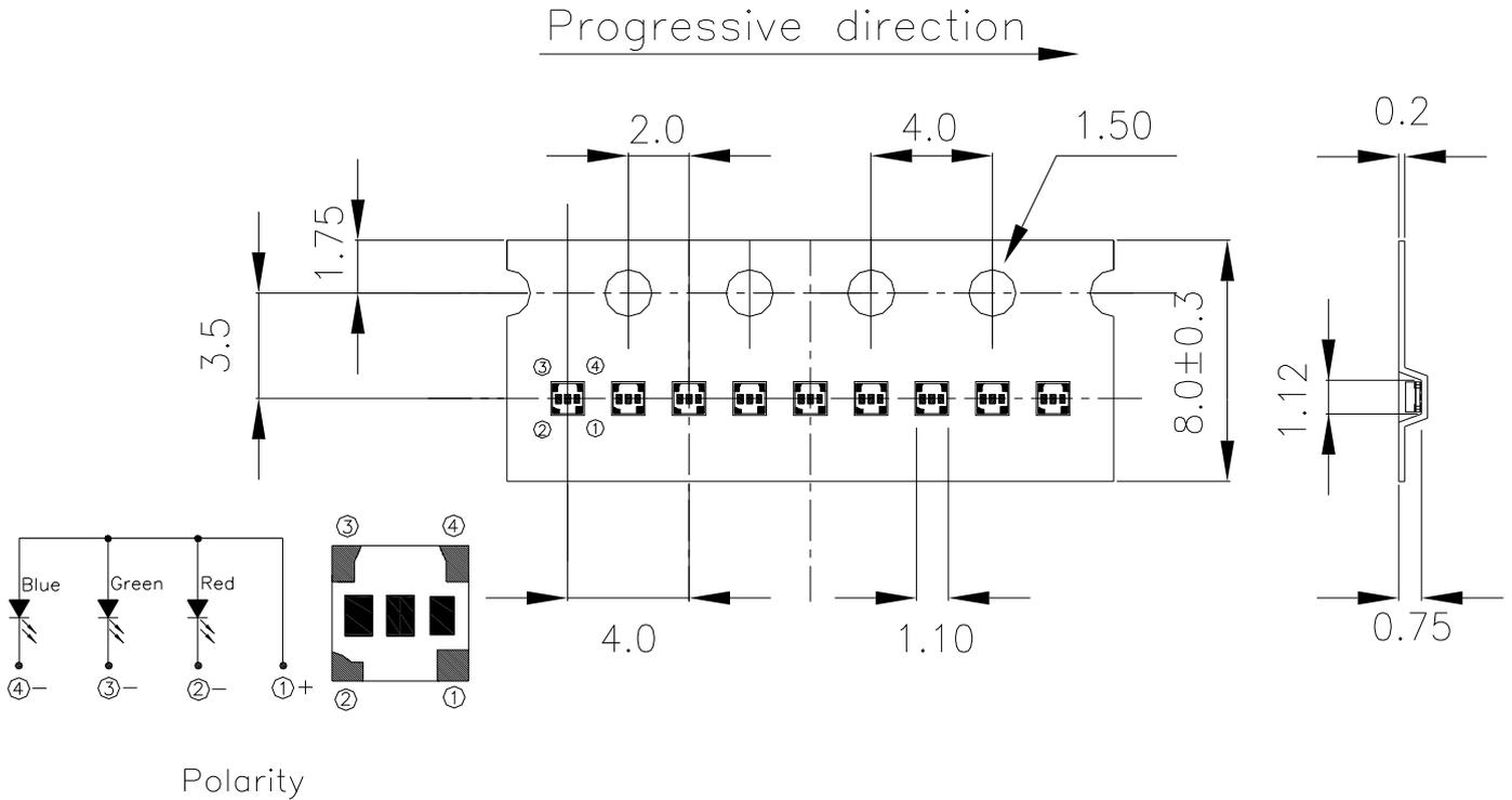
Note: Tolerances unless mentioned  $\pm 0.1\text{mm}$ . Unit = mm
