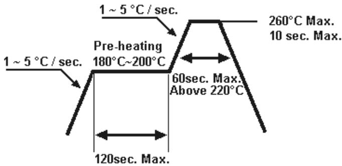
4.2.2 Reflow soldering should not be done more than three times.
